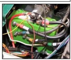
• Connect battery negative cable - Tighten w/10mm wrench or socket per specs on page 10.
